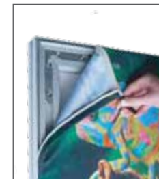
Insert the fabric by pushing the silicone strip into the channel of the extrusion.
